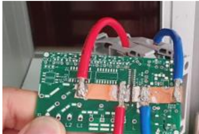
Figure 17: Thermal test board (bottom)
